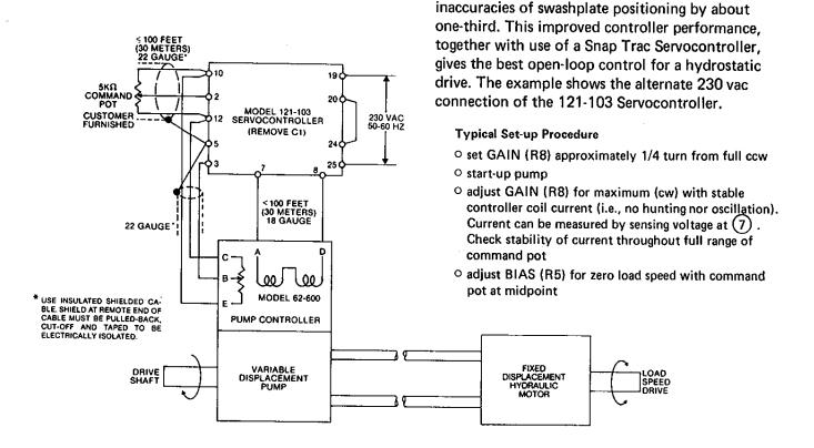
The electrical feedback pump controller reduces
