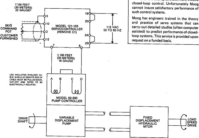
Moog's pump controller uses a dc control signal. When 115 vac is available, the Model 121-103 Snap Trac Servocontroller provides a convenient drive circuit for the pump controller. The stabilized power supplies and current feedback of the 121-103 eliminate unwanted control signal variations. The external velocity command pot can be located in an operator's control console.
